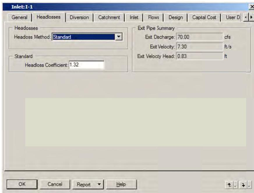
**Figure 14** - Type in “1.32” for the headloss coefficient.
